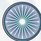
0 Lead – Material is thrown straight and gives insufficient separation
